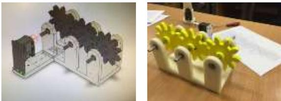
CAD Design of Gear Test Rig (on the left) and 3D Printed Gear Test Rig (on the right)
