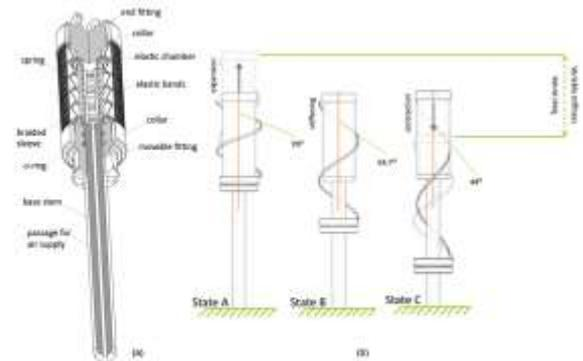
(a) Schematics of the bi-directional muscle. (b) Working concept of the bi-directional muscle. A single braid fiber is shown instead of the whole braided sleeve for clarity.
