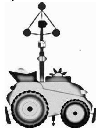
Mobile landmark mounted on a small robot
