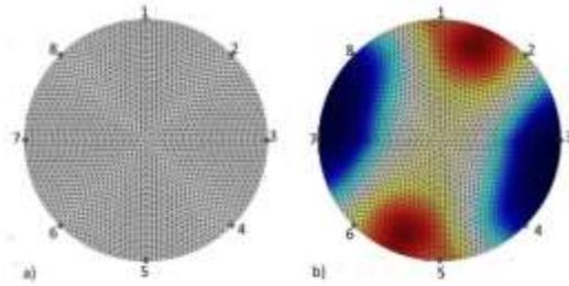
On the left, the Finite Element Model of the sensor. On the right, the simulated reconstructed image when pressure is applied simultaneously at two opposite points near electrode pairs 1-2 and 5-6 (in red).
